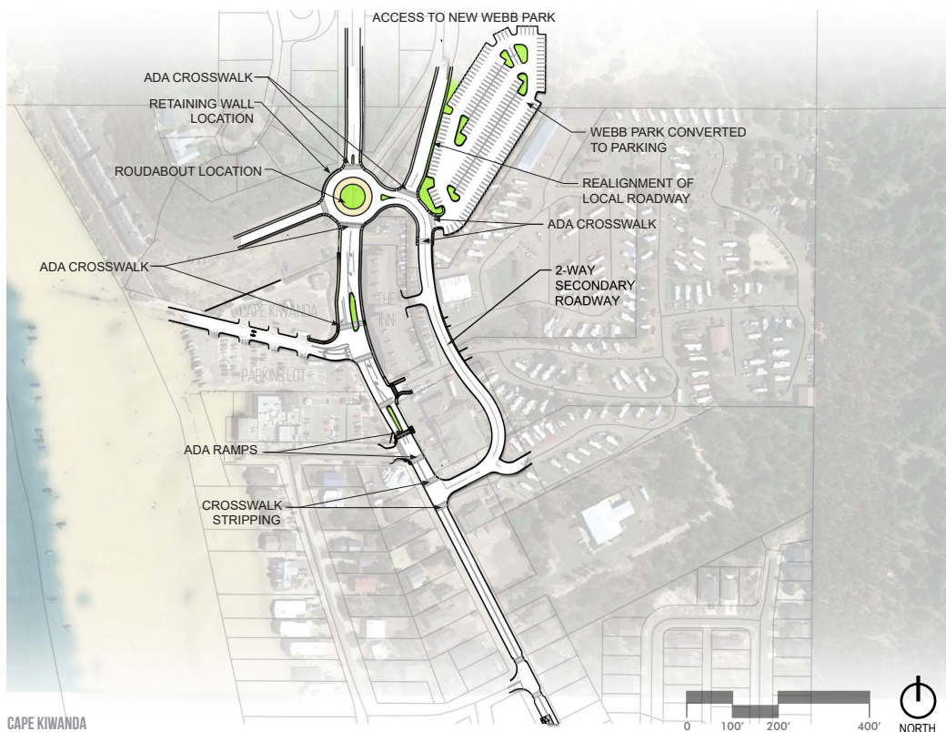
Figure 5. Roundabout and Backage Road
