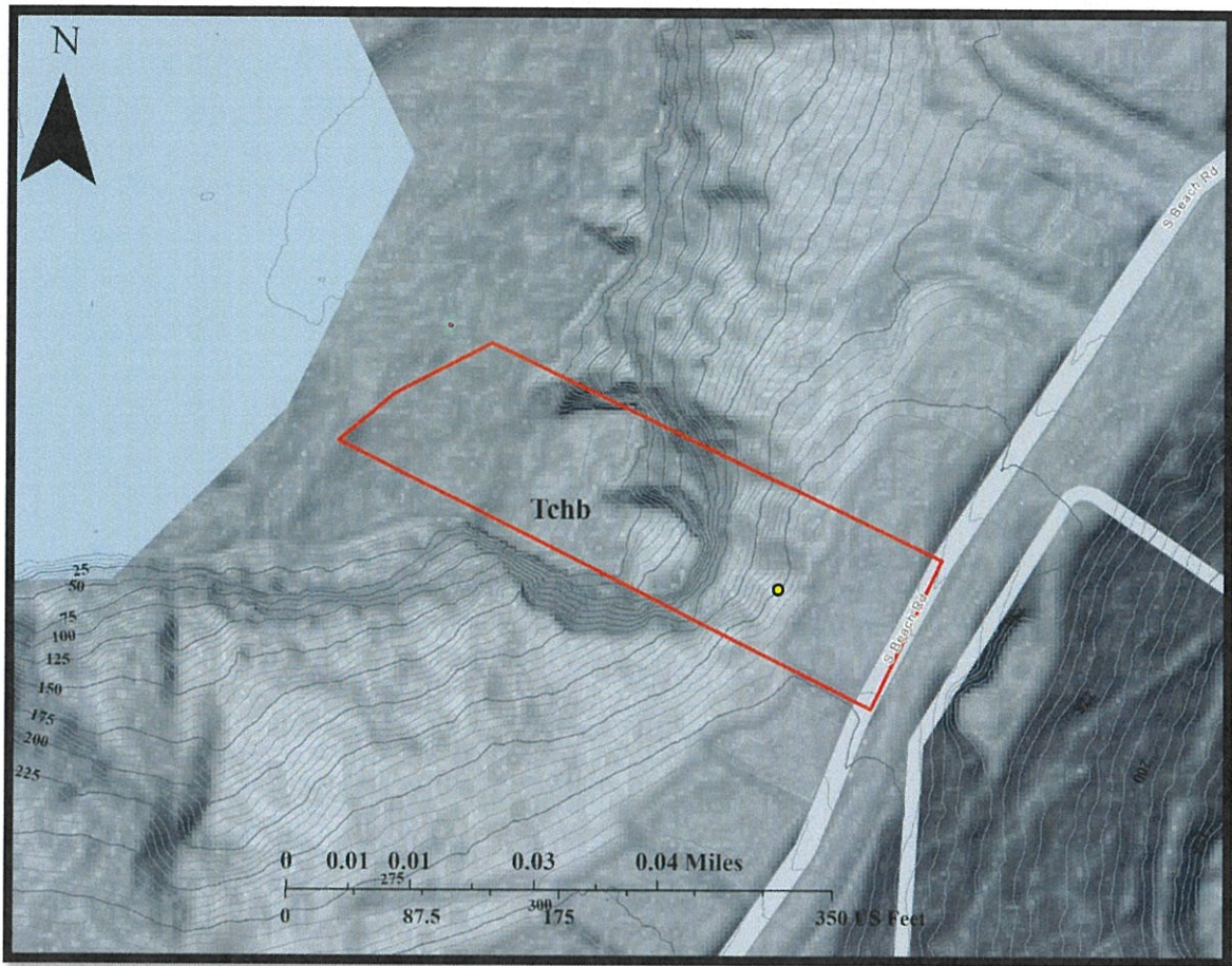
Figure 3: Geologic map of the area (source: DOGAMI OGDC-7). Subject tax lot outlined in red; approximate location of Sitka Spruce notated as a yellow point; Tchb: Tertiary Basalt of Cascade Head; Contour interval = 5 feet
